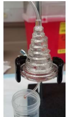
Figure 3: Mounted LRS Chamber. Chamber mounted, drained of contents, and washed with 100% plasma.
